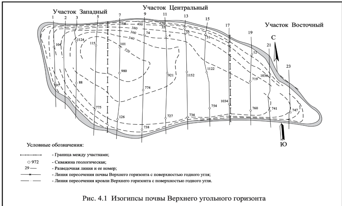
Figure 4-1: Plan showing the geological structure and depth of the Shubarkol Deposit taken from Figure 4.1 in the 2014 TEO Update Report
