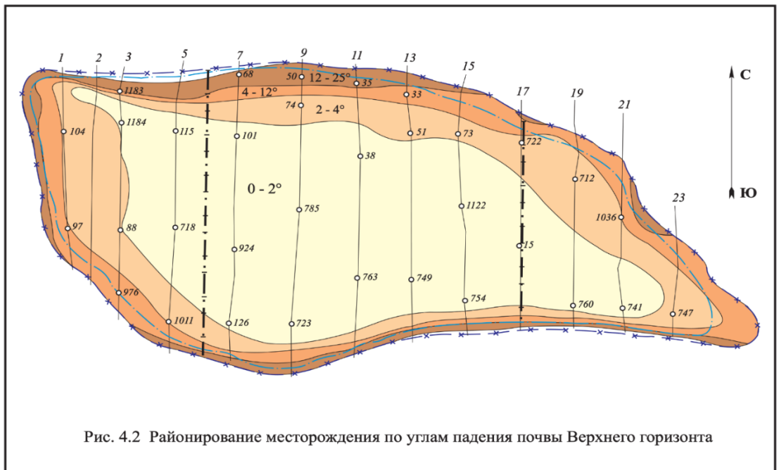
Figure 4-2: Plan showing the geological structure and strata dip of the Shubarkol Deposit taken from Figure 4.2 in the 2014 TEO Update Report
