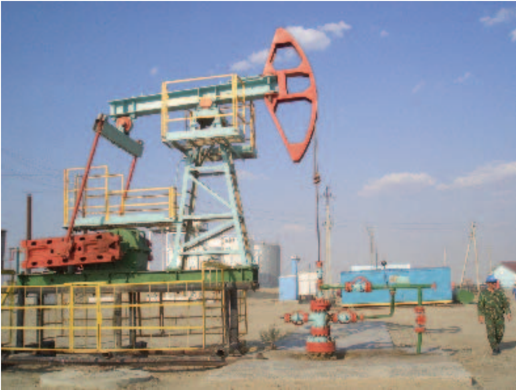
DossorMunaiGas NGDU Botakhan Field Sucker-Rod (Beam) Pump Oil Well
