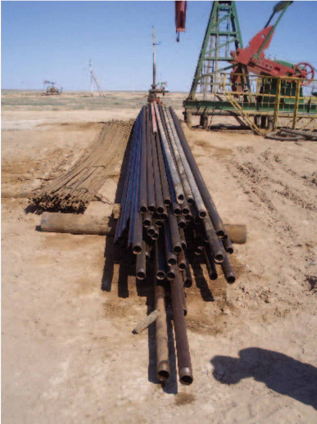
MakatMunaiGas NGDU East Makat Field Tubing and Rods Pulled for Repair and Maintenance
